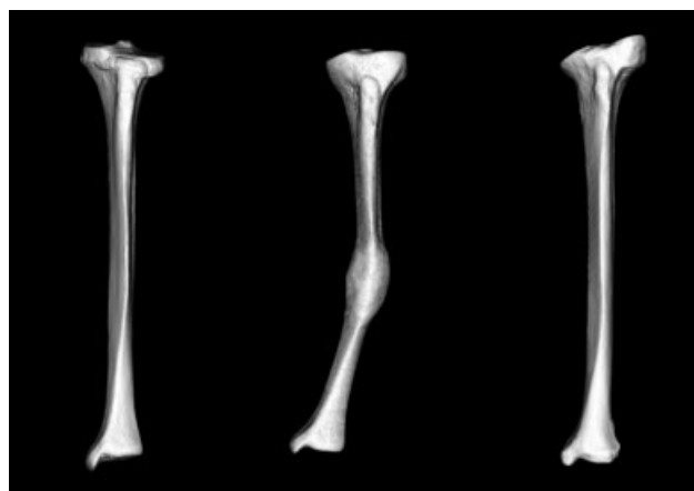
Figure 3. The three types of deformed phantoms used in our laboratory study. Approximate deformities were: (left) 10° valgus with 30° internal rotation; (middle) oblique deformity 15° varus with 10° procurvatum; (right) 30° varus
